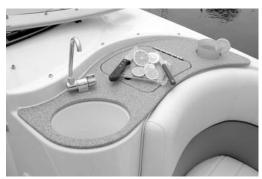
Figure L-2: Integrated Sink, Cooler & Trash Receptacle
