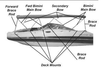
Figure O-2: Forward Bimini & Bimini Top
