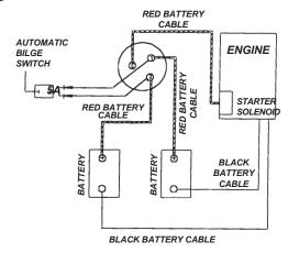
Figure H-2: Single Engine-Dual Battery Installation
