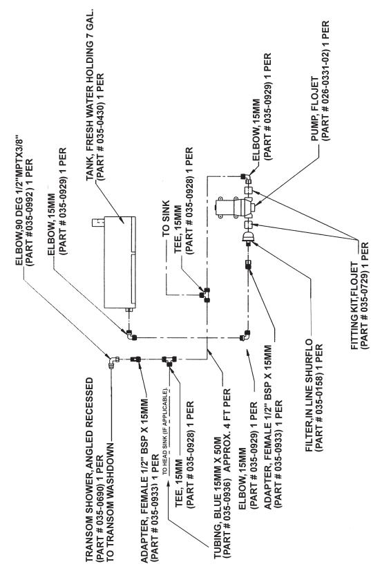
Figure J-12: General Water System Diagram
