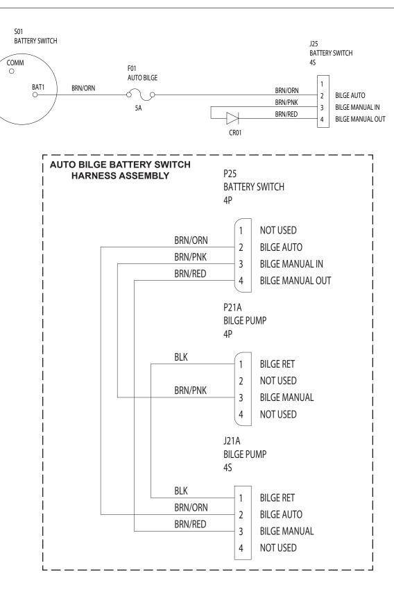
244/274 (234/264) FUNSHIP CE - SINGLE BATTERY SWITCH SHUTOFF PANEL ASSEMBLY
