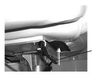
Lift adjustment lever up to move forward and back.
