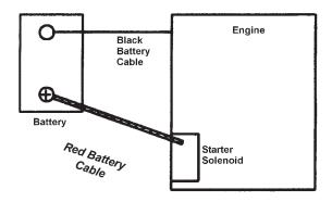
Figure H-1: Single Engine-Single Battery Installation
