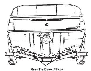
Figure S-12: Rear Tie Down Straps
