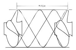
Figure E-1: Propeller Pitch & Diameter
