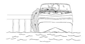
Figure B-6: Minimize Exhaust Re-enty
