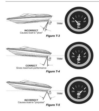
Figures T-3-T-5: Trimming the Boat with Outdrive
