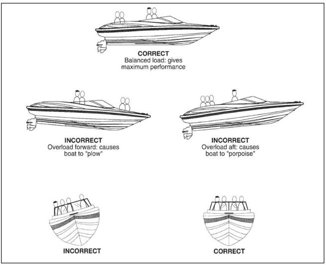
Figure T-1: Loading Passengers and Gear
