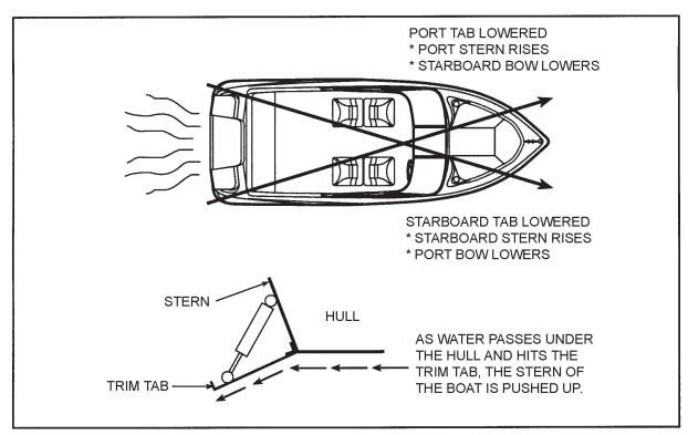
Figure T-2: Trimming the Boat with Trim Tabs
