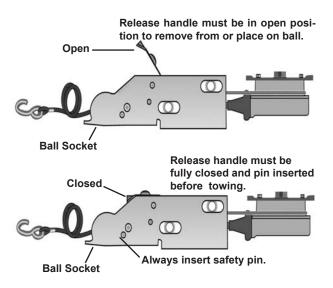
Figure S-7: Surge Brake Actuator & Coupling Assembly
